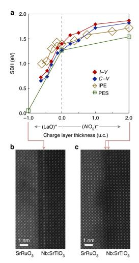
**Figure 4 | Summary of the SBH tuning. (a)** SBH values obtained from *I*-*V*, *C*-*V*, IPE and PES measurements plotted as a function of interlayers,  $(LaO)^+$  and  $(AIO_2)^-$ . (**b,c**) High-angle annular dark-field-STEM images of SrRuO<sub>3</sub>/Nb:SrTiO<sub>3</sub> heterointerfaces with (**b**) 1u.c.  $(LaO)^+$  and (**c**) 2 u.c.  $(AIO_2)^-$  insertions.
