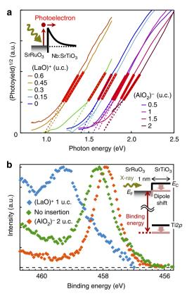
Figure 3 | Photoelectric measurements of the SBH. (a,b) IPE and PES spectra for SrRuO<sub>3</sub>/Nb:SrTiO<sub>3</sub> Schottky junctions with (LaO)<sup>+</sup> and (AlO<sub>2</sub>)<sup>-</sup> insertions. Red lines in **a** show the region over which the linear extrapolation (dashed lines) was carried out. Insets show the schematics of each measurement. The black arrow in **b** represents the detection width (~1nm).
