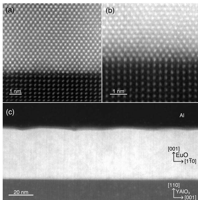
FIG. 1. Cross-sectional HAADF-STEM images of epitaxial EuO films grown on YAlO<sub>3</sub>, viewed along the [110] zone axis of the EuO film and the [1 $\bar{1}$ 0] zone axis of the YAlO<sub>3</sub> substrate. (a) Undoped EuO grown by adsorption control at 400 °C and (b) ~5% La-doped EuO grown under flux-matched conditions at 250 °C. (c) Low-magnification view of (b) depicting the entire film. The interfaces are coherent and chemically abrupt.
